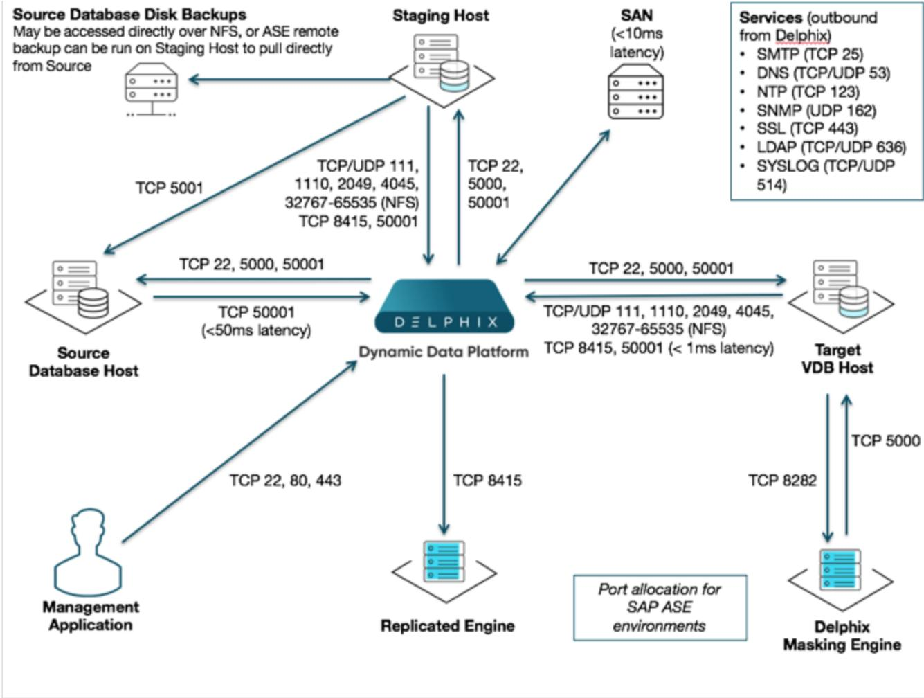
Delphix stays in sync with source databases by monitoring the ASE backup server log. When it sees a new database dump or transaction log has been created, it attempts to load it into the ASE staging instance.
